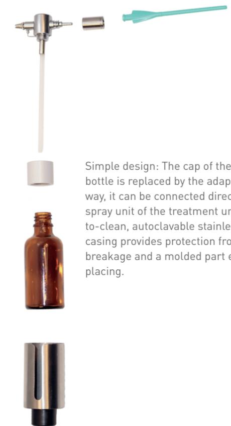
Simple design: The cap of the pharmacy bottle is replaced by the adapter. In this way, it can be connected directly to the spray unit of the treatment unit. An easy-to-clean, autoclavable stainless steel casing provides protection from glass breakage and a molded part enables safe placing.
