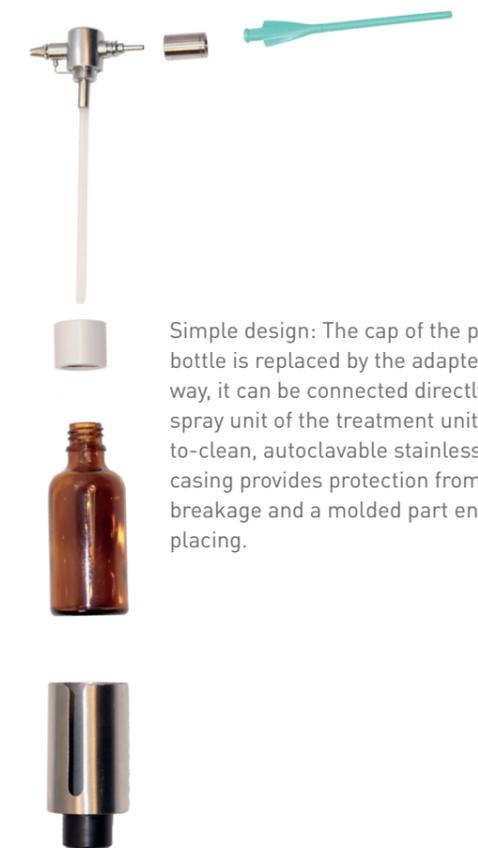
Simple design: The cap of the pharmacy bottle is replaced by the adapter. In this way, it can be connected directly to the spray unit of the treatment unit. An easy-to-clean, autoclavable stainless steel casing provides protection from glass breakage and a molded part enables safe placing.
